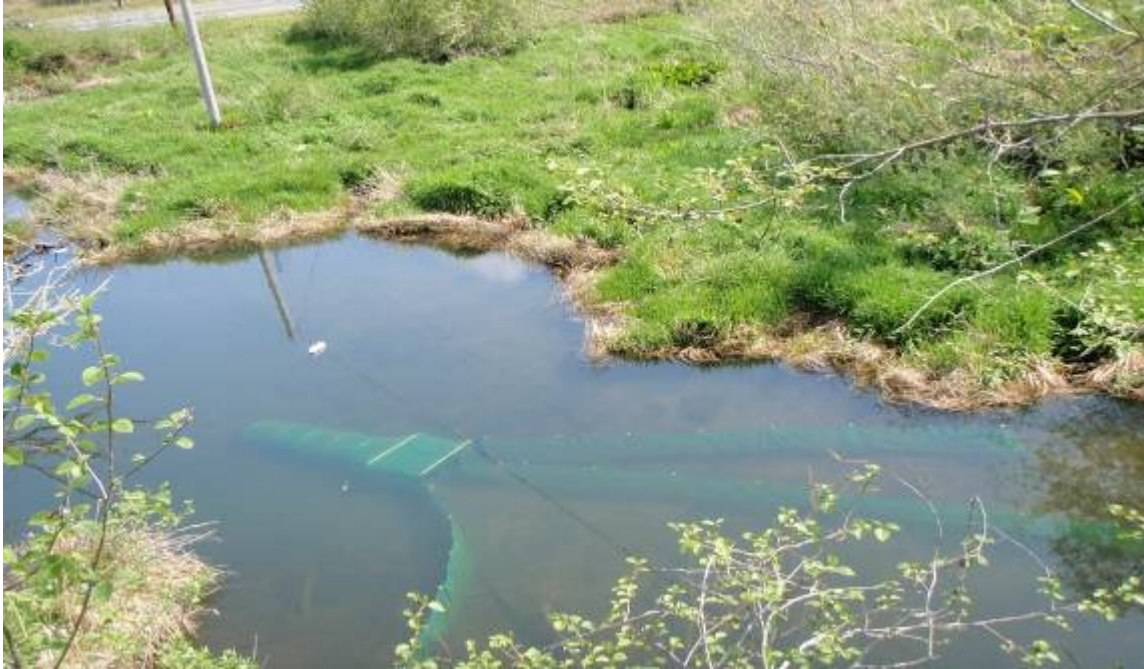
Figure 12. A three-foot by four-foot hooped fyke net with lead block net (3 ft x 50 ft) and two wing block nets (3 ft x 50 ft) set in Panther Creek Pond, Lower Klamath River Sub-basin.
