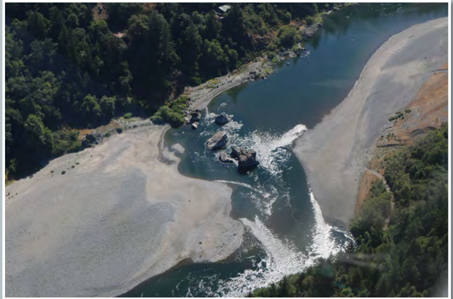
Sedimentation & development of extensive river bars combined with low flow releases from the dams made the Klamath River nearly impassible in 2016
