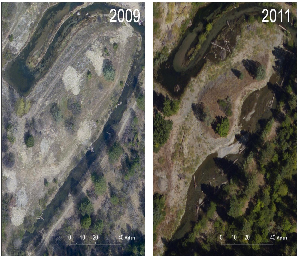
Figure 9. Aerial views of Cemetery Side Channel (rkm 175.75) prior to construction in 2009 (left photo) and post construction, post two high flows in 2011 (right photo). Both photos were taken at summer base flow ~12.7 cms (450 cfs).
