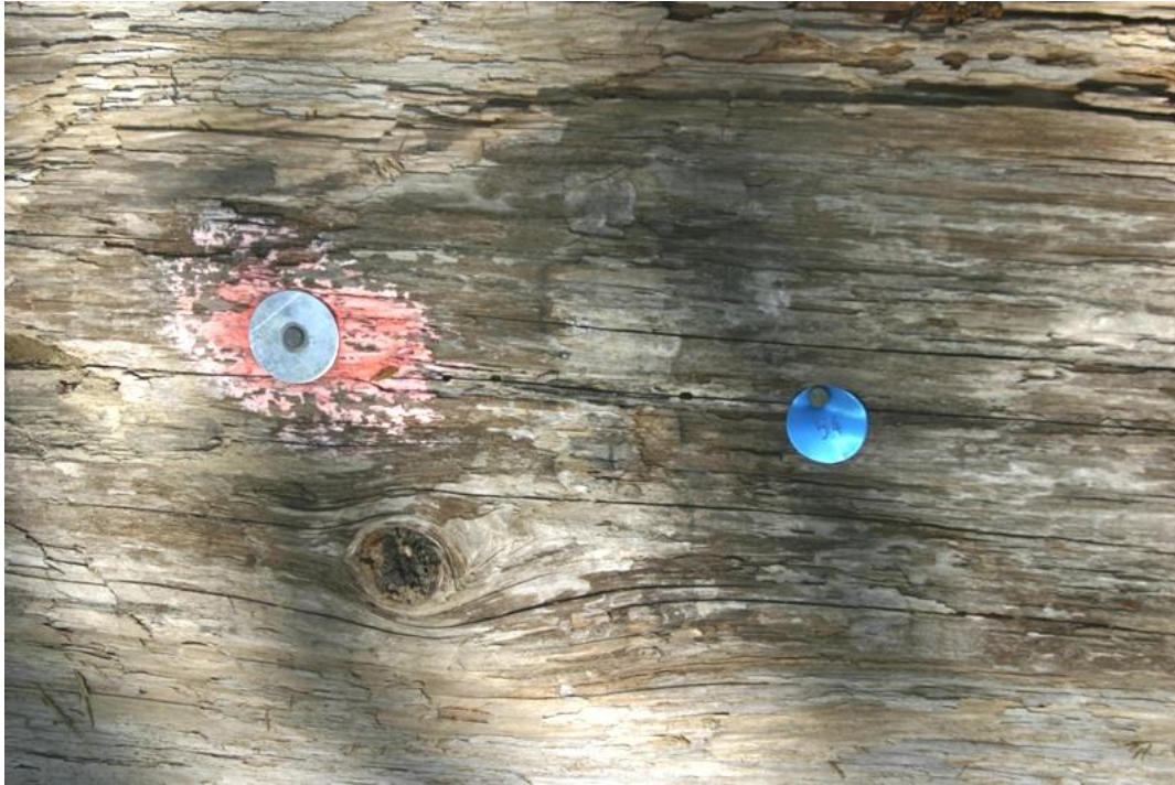
Figure 116. Sequentially numbered tree tag (right) and survey pin (left) installed in a piece of placed LWD, McGarvey Creek, Lower Klamath River, California, 2007.
