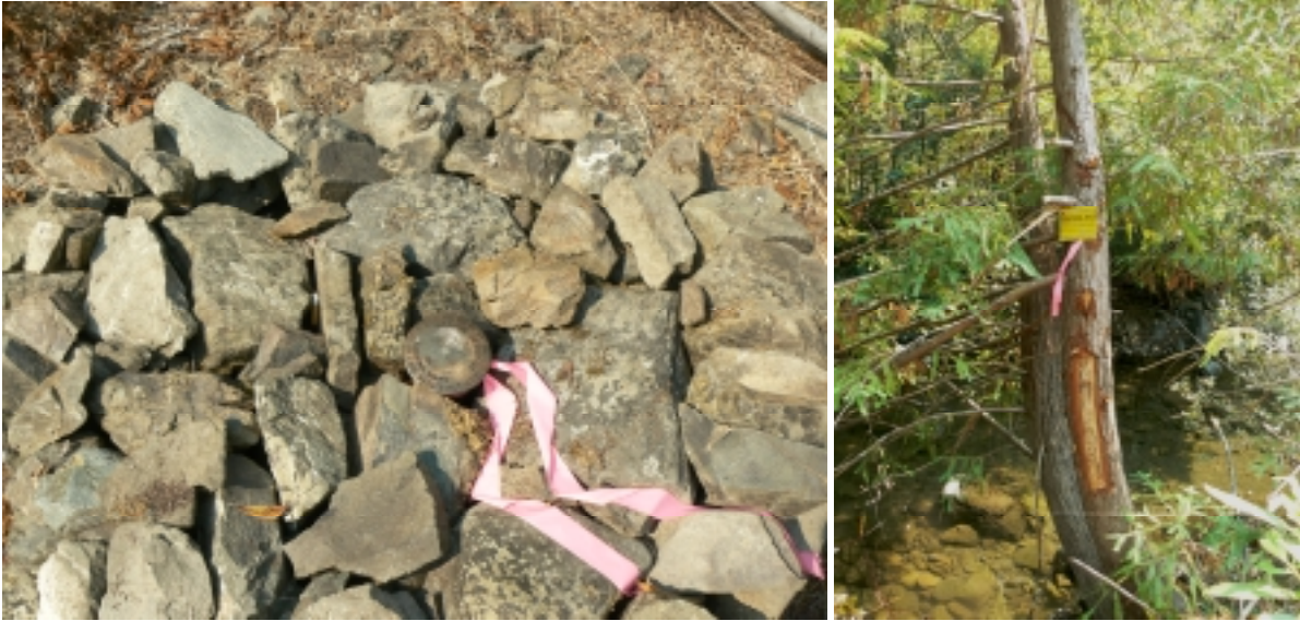
Figure 18. Photographs of a permanent bench mark (Left Photograph) and a survey bearing tree (Right Photograph) established in 2008 by Yurok Land Management survey crews in Tectah Creek, Lower Klamath River Sub-basin, California (September 2008).
