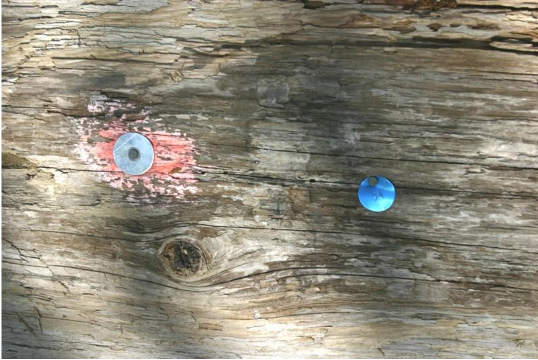
Figure 97. Sequentially numbered tree tag (right) and survey pin (left) installed in a piece of placed LWD, West Fork McGarvey Creek, Lower Klamath River, California, 2007.
