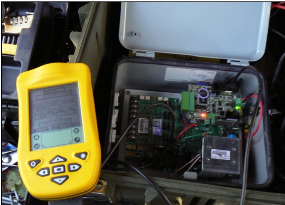
Figure 14. Multiplexer datalogger and handheld PDA used at all remote Passive Integrated Transponder (PIT) tag monitoring systems in McGarvey Creek.
