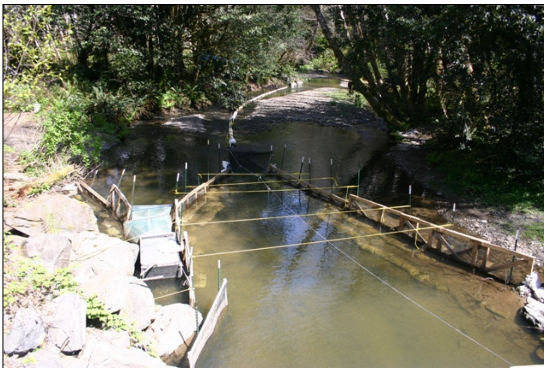
Figure 10. Pipe/frame net outmigrant trap deployed in McGarvey Creek, 2008.
