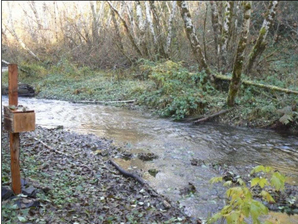
Figure 13. Looking downstream at Lower McGarvey pass-through antenna and housing box for tuning capacitor.
