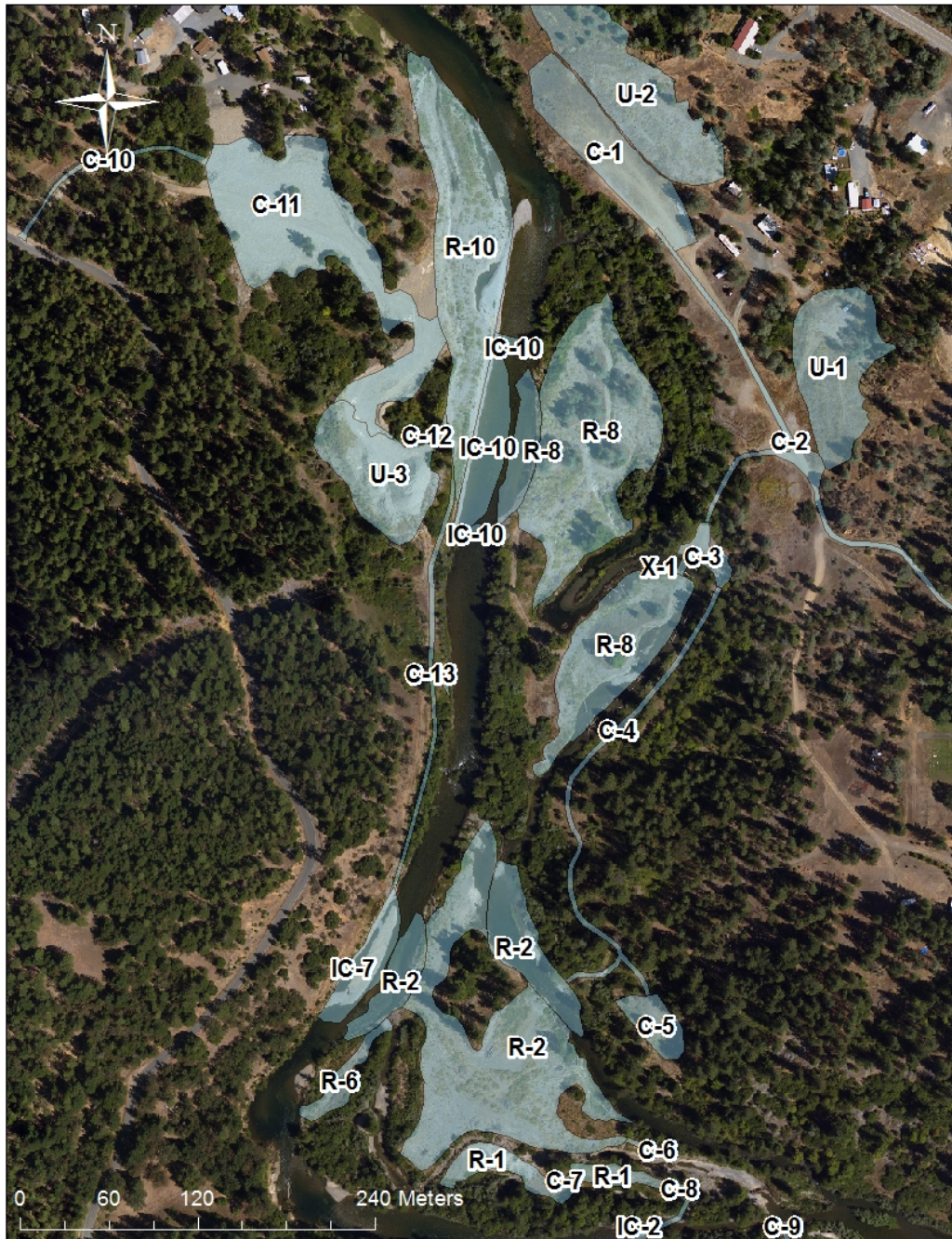
Figure 2. Aerial photos of Sawmill rehabilitation site design elements taken in 2011. Blue polygons indicate design rehabilitation site design elements (HVT and McBain and Trush 2009). 'IC' indicates an in-channel feature, 'R' is a riverine/floodplain feature, 'C' indicates contractor use areas, 'U' identifies spoil locations and 'X' is a construction crossing.
