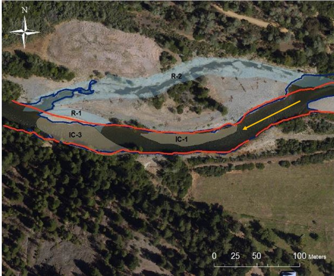
Figure 18. Aerial photo taken in 2011 of the Trinity House Gulch rehabilitation site (rkm 167.5-167.9). IC-1 and IC-3 were designed point bars constructed in 2010. R-1 was a designed river meander and R-2 was a designed low flow side channel also constructed in 2010. The red lines represent pre-construction wetted edge surveyed in 2010 at 14.3 cms (505 cfs). The blue lines represent post-construction wetted edge surveyed in 2011 at 13.6 (480 cfs). The orange arrow indicates flow direction.
