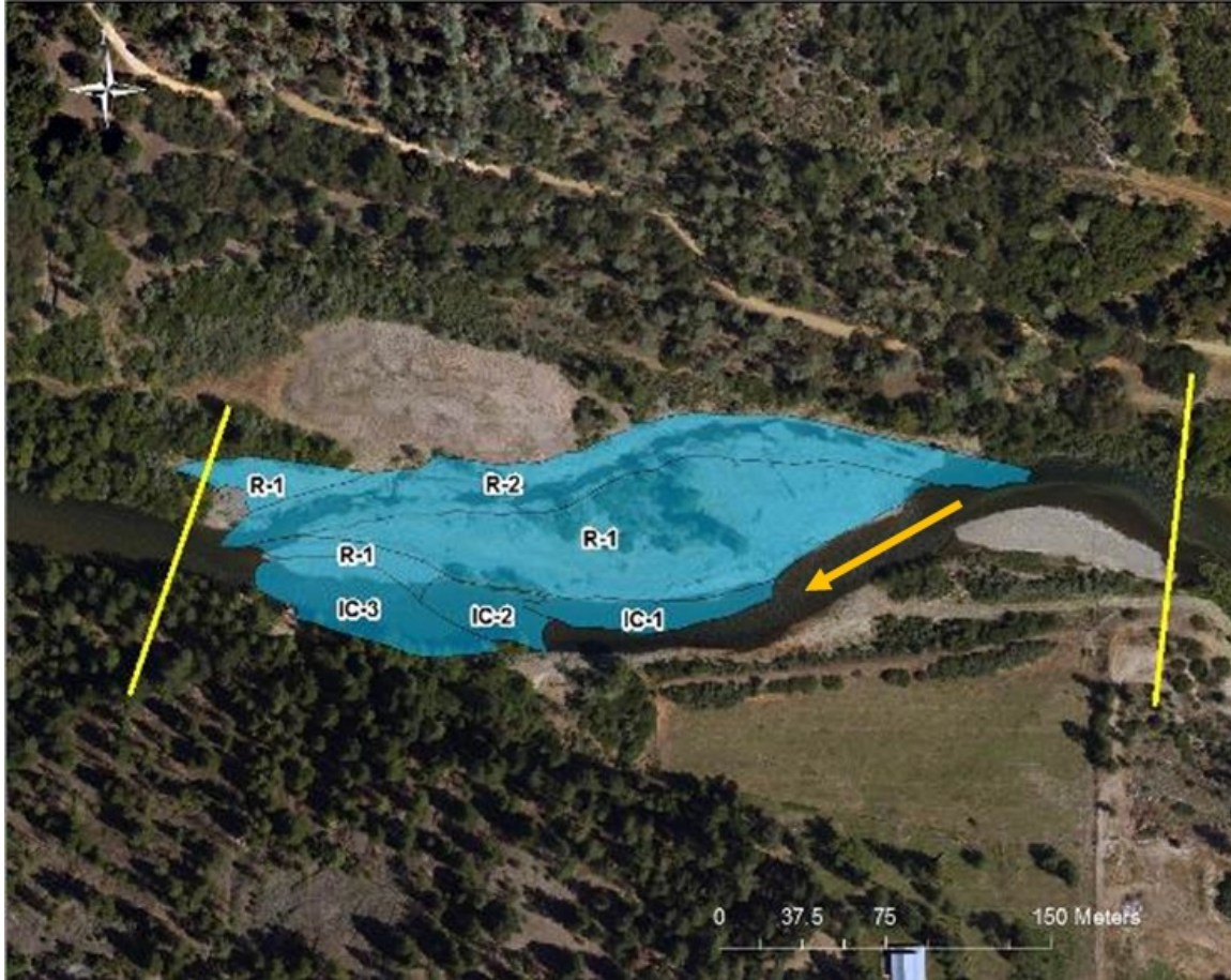
Figure 4. Aerial view of Trinity House Gulch rehabilitation site design elements and habitat survey extents. Yellow lines indicate pre- and post-construction summer base flow mapping extents. The orange arrow indicates flow direction.
