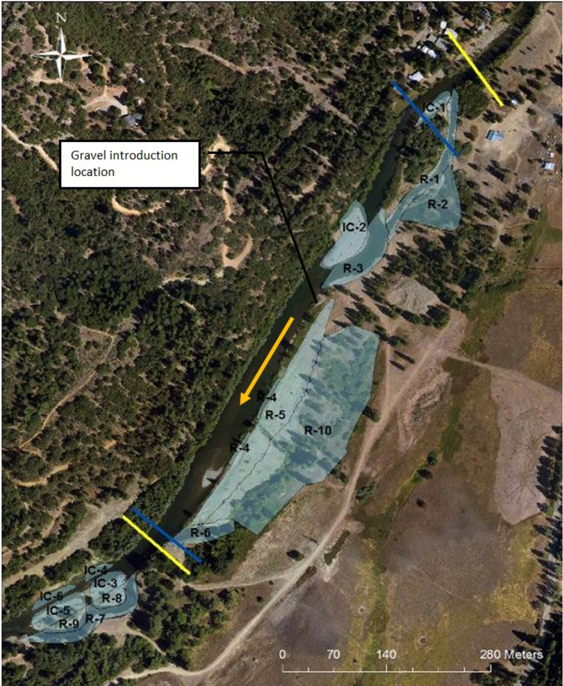
Figure 2. Aerial view of Lowden Meadows rehabilitation site design elements and habitat survey extents. Yellow lines indicate pre- and post-construction winter base flow mapping extents. Dark blue lines indicate pre- and post-construction multiple flow to habitat mapping extents. The orange arrow indicates flow direction.
