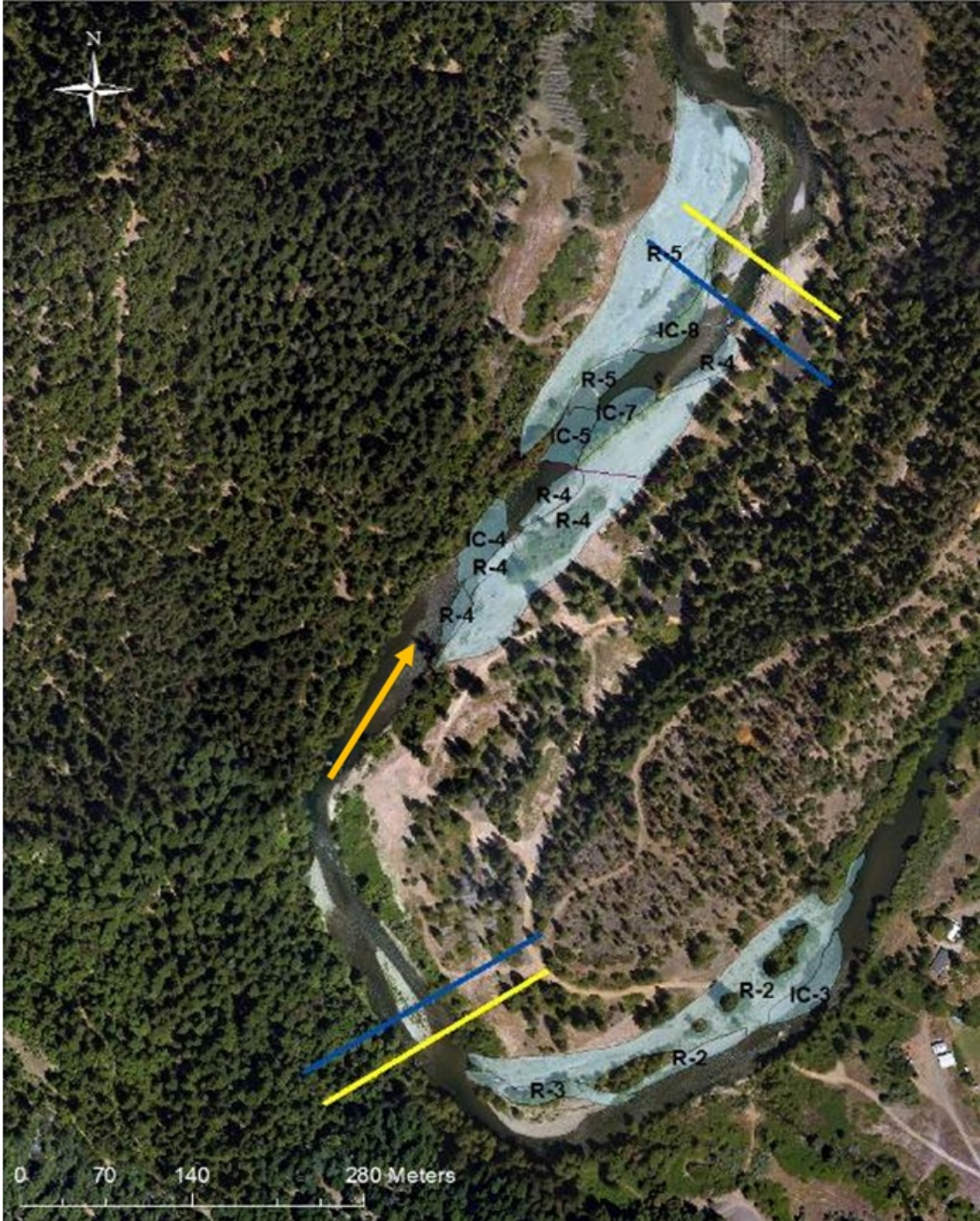
Figure 3. Aerial view of Reading Creek rehabilitation site design elements and habitat survey extents. Yellow lines indicate pre- and post-construction winter base flow mapping extents. Dark blue lines indicate pre- and post-construction multiple flow to habitat mapping extents. The orange arrow indicates flow direction.
