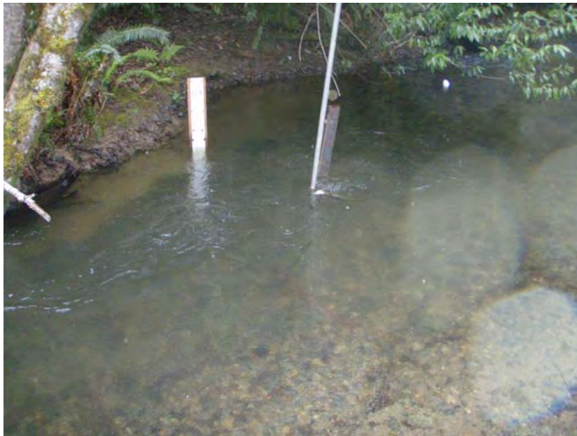
Figure 3. McGarvey Creek gaging station turbidity boom and staff plate (downstream of turbidity boom on left bank).
