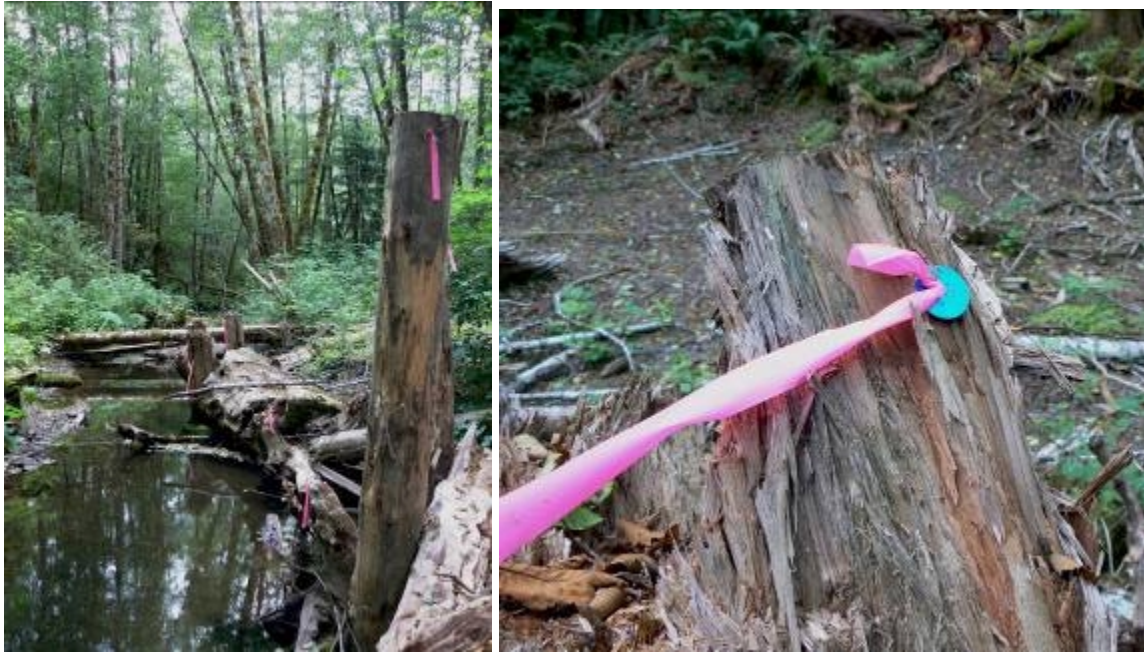
Figure 4. Photographs of complex wood jams constructed in Waukell Creek in summer 2009 and the numbered ID tags surveyed to document any movement of wood over time.
