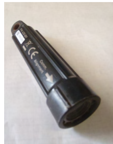
Figure 9: Left: Water monitoring locations established in 2012. All locations displayed are covered in this report excluding the Turwar Creek Alcove (TWA). Right: HOBO U22 continuous water temperature logger
