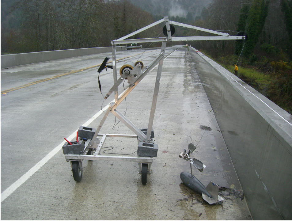
Figure 7. Photo of bridge crane mounted flow measuring equipment at Highway 169 bridge crossing at Lower Turwar Creek, December 27, 2007.
