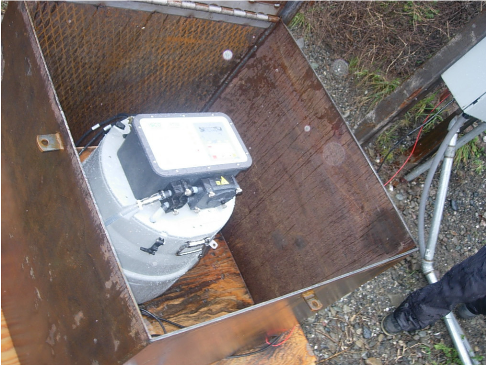
Figure 5. Photo of automated pump sampler used to collect unattended water samples to be analyzed for suspended sediment concentrations, Lower Turwar Creek, WY 2008.
