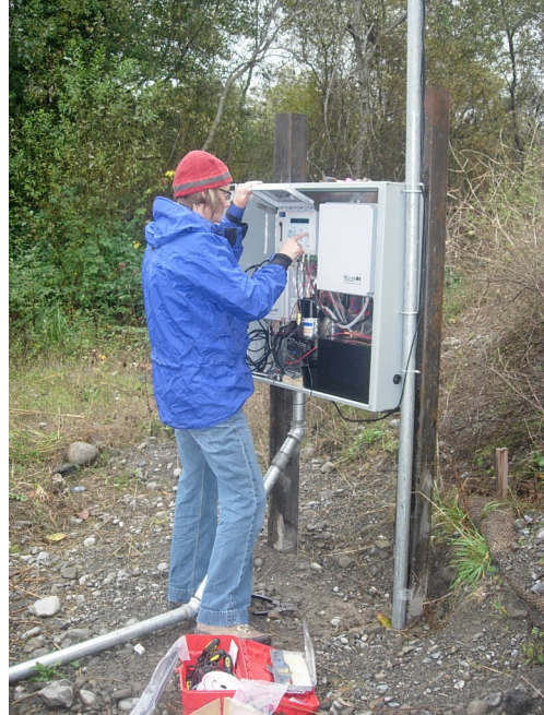
Figures 2 and 3. Photo of Lower Turwar Creek Monitoring Station and Monica Hiner programming the datalogger.
